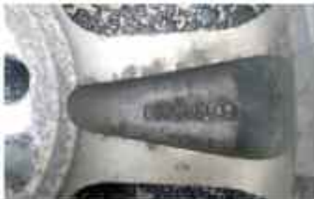
This is a 45 mm offset. It is often, but obviously not always, accompanied by an "ET" marking.
