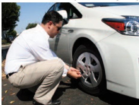
A vehicle with a recommended inflation pressure of 35 psi running 20%, or 7 psi, below recommended pressure will result in a 10% increase in rolling resistance - which translates into a 1.5% decrease in fuel mileage.
